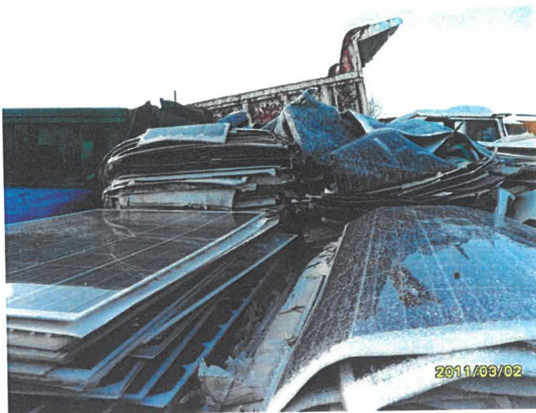
Figure 4: The mangled PV panels in this picture illustrate the nature of broken solar panels; the glass cracks but the panel is still in one piece. Image Source: http://img.alibaba.com/photo/115259576/broken_solar_panel.jpg
