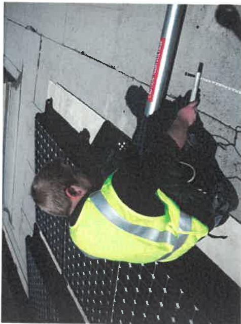
Figure 3-26 Rooftop DC Cable Conduit - Static Magnetic Field Measurements
