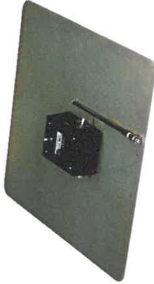
Figure 4-3 AH Systems Model SAS-550-1B Active Monopole Antenna - For measurement of electric field strengths in the range of 9 kHz to 60 MHz. The telescoping rod element is extended and connected to the BNC connector on the top of the electronics box in the center of the ground plane during measurements.
